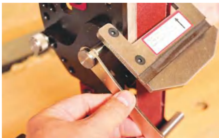
▲ The captive spanner is used to lock off the toolrest
